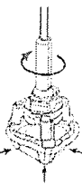
Figure 10: Rotate the valve holder handle to deflect the mitral stent posts inward.
